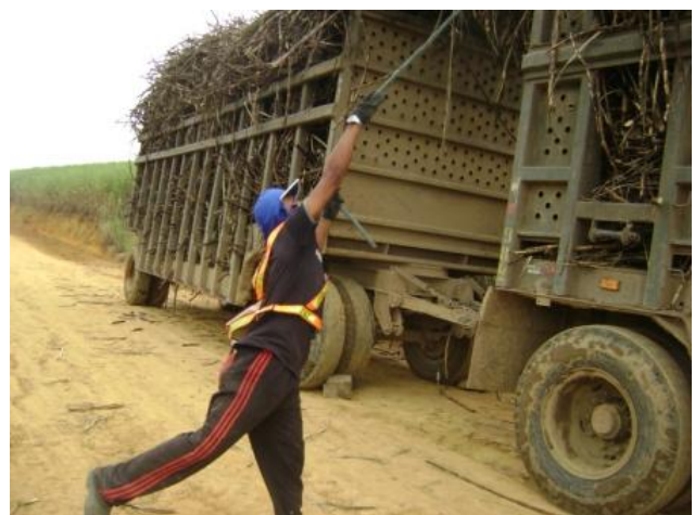
Figure 2. Lashing of cane cargo in the truck or in the trailers, by means of ropes thrown over the load (working activity 1)
