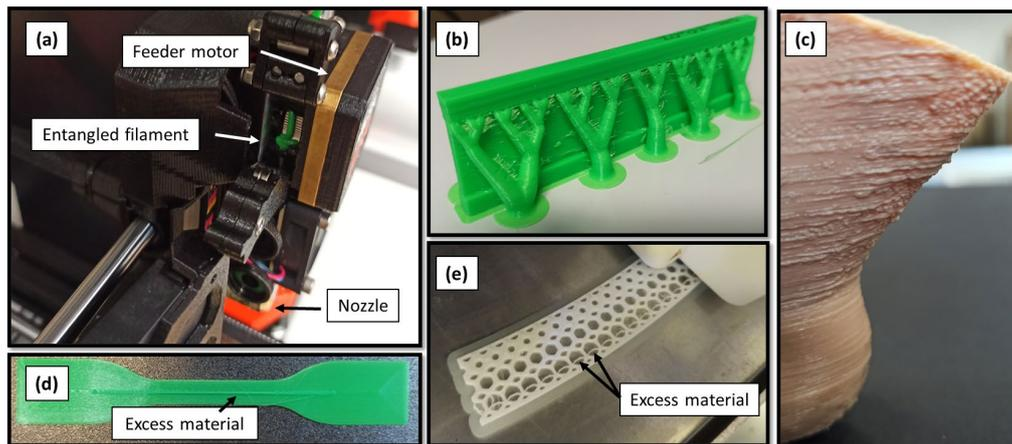
**Figure 2:** Examples of most common issues found when 3D printing TPUs: (a) Filament entanglement inside a direct drive extrusion system of a Prusa Mk4; (b) Stringing effect using Flexfill TPU 92A; (c) Material blobs in a part made of Filaflex 95A; (d) Accumulation of excess material in a tensile specimen produced with a concentric infill pattern; (e) Excess material deposited with a pattern when producing a cellular structure.
