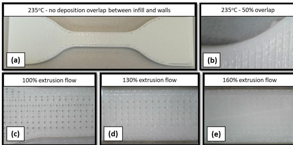
**Figure 4:** Samples of tensile specimens produced with TPU 95A in the Ultimaker S5: (a) Representation of lack of material generating gaps between infill and walls; (b) Amplified view of a specimen produced with overlap between infill and walls; (c)-(e) Amplified view of equivalent samples produced with variable extrusion flow.
