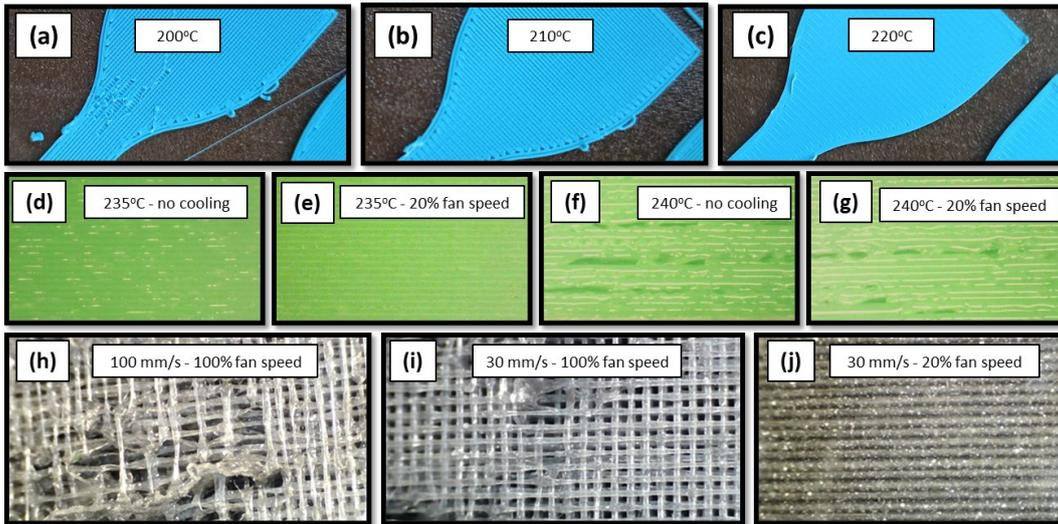
**Figure 3:** Amplified views of specimens produced in a Prusa Mk4 with: (a)-(c) Smartfil TPU 93A; (d)-(g) Flexfill TPU 92A; (h)-(j) Flexfill TPU 98A.
