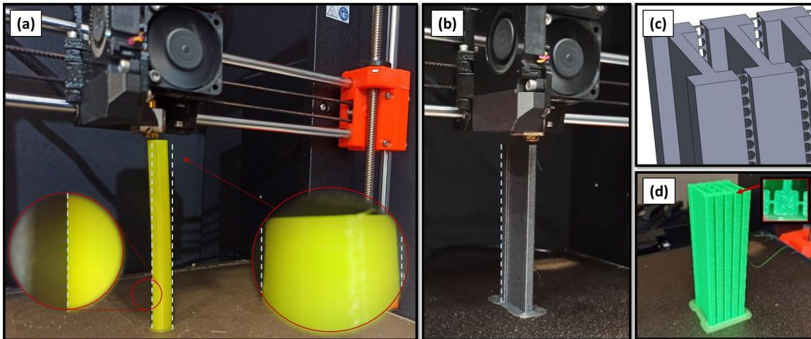
**Figure 5:** Examples of the instability while printing tall and slender structures: (a) Tower of Smartfil TPU 93A with differences in geometrical accuracy caused by wobbling; (b) Test specimen of Flexfill TPU 98A; (c) CAD model of the very thin sacrificial grid connecting specimens; (d) Five connected specimens of Flexfill TPU 92A.
