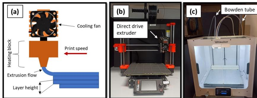
**Figure 1:** Fused filament fabrication process: (a) schematic illustration of relevant process parameters; (b) a direct drive extrusion machine, Prusa Mk4; (c) a Bowden-based extrusion machine, Ultimaker S5.
